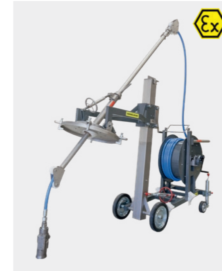
Lance hose system The lance is positioned over the manhole by the mobile chassis. The lance can be manually rotated, swivelled, retracted and extended.
