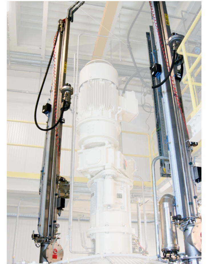
Lance system - moved and actuated pneumatically
