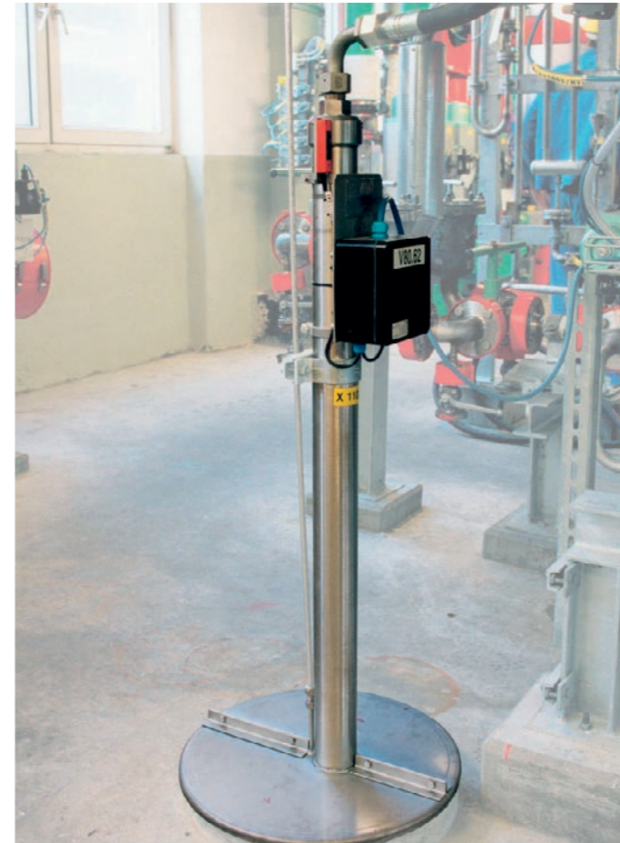
Lance system - moved hydraulically/pneumatically actuated
