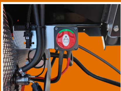
Main battery switch
